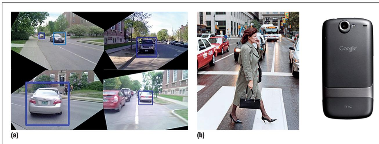
**Figure 2.** The WalkSafe app (a) offers real-time detection of the front and back views of cars, noting when a car is approaching or moving away from a user on the phone. (b) Each video frame is preprocessed to compensate for the phone tilt.
