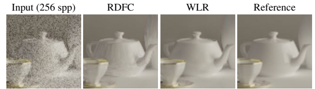
Figure 4: Comparison of RDFC and WLR on the DINING ROOM scene. The Joint NL-Means filter used by RDFC can only combine pixels with similar values, which leaves residual noise on the curved teapot surface, where the normals change rapidly. In contrast, WLR uses a first-order regression that better models the data, leading to smoother results.
