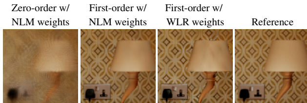
Figure 6: Using the same NL-Means regression kernel as in Figure 2 with zero- and first-order regressions. Even though this kernel gives a poor result in a zero-order regression, it produces a high-quality result when paired with a first-order regression, comparable to the WLR output, despite using a much simpler weighting scheme.
