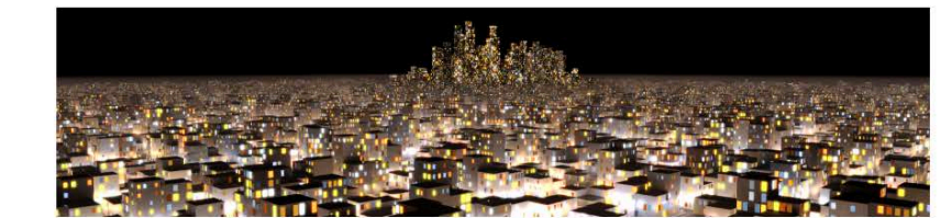
Fig. 1. A procedural city with 363,036 lights, one GI bounce and participating media. Rendered with 16 samples per pixel, each shading point takes an average of 7 shadow rays (45 for the volume integral). We shoot an average of 1700 rays per pixel. The image rendered in 20 minutes on a quad core Intel i7.
