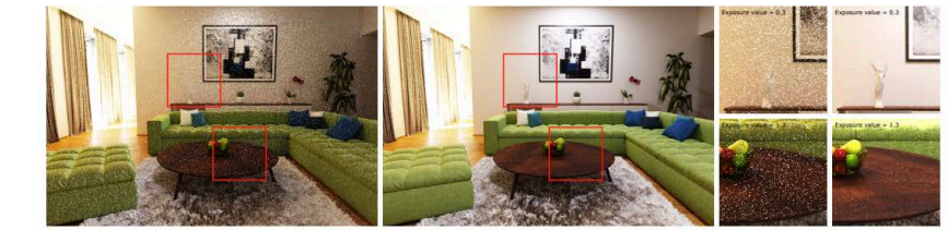
Fig. 1. Equal-time comparison (60 s) of path-traced global illumination solutions computed using our learning-based direct illumination sampling method (right) and a baseline sampling method without learning (left). While both methods start off by sampling lights proportionally to rough estimates of their unoccluded contribution, our method progressively incorporates information about their actual contributions, including visibility, dramatically reducing image variance.
