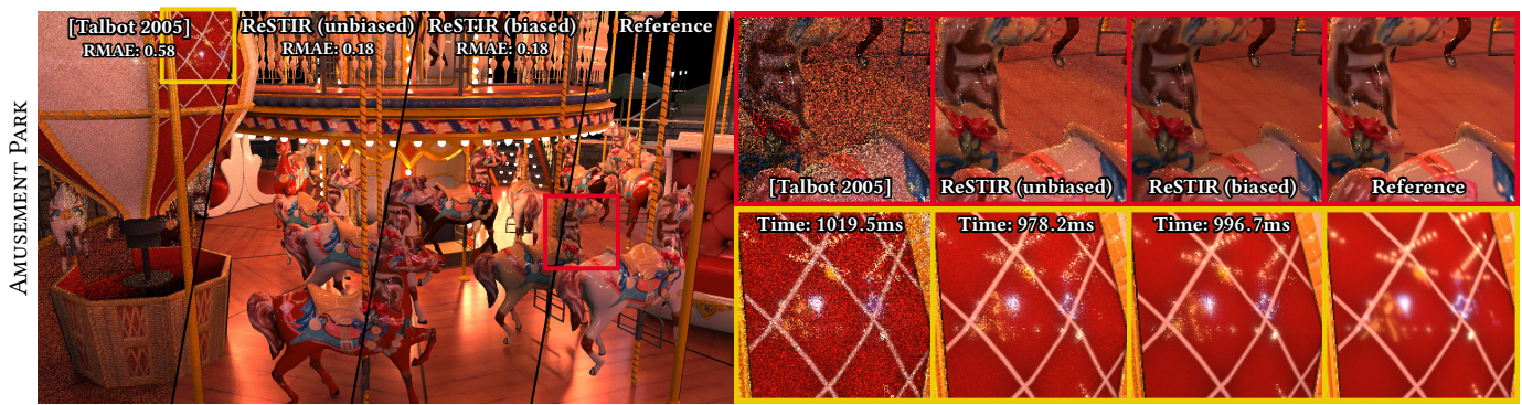
Fig. 10. An equal time comparison given a longer 1s compute budget. We compare a streaming implementation of Talbot et al. [2005] with our biased and unbiased spatiotemporal sample reuse. Our AMUSEMENT PARK scene has 3.4 million dynamic emissive triangles. Carousel ©carousel_world
