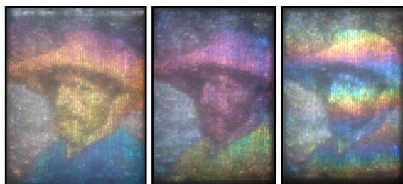
Figure 14: Misalignments of the masks compared to a proper alignment (left). A positional misalignment causes a color shift similar to a hue shift (middle). Rotational misalignments varies the hue shift over the projection (right).
