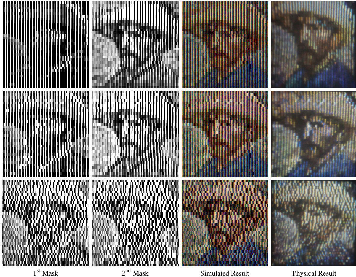
Figure 13: A series of experiments showing the first masks (left), the second masks (middle left), simulated results (middle right) and a photograph of the actual projections with optimized masks (right). The top row applies masks that double the light throughput, the middle row triples the light output and the bottom row shows the result of obfuscated masks.
