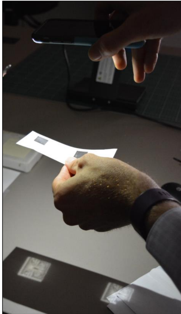
Figure 1: The PBI feature. The lens array, applied to polymer substrate is illuminated by an iPhone 6s flash. The projected image can be clearly resolved.
