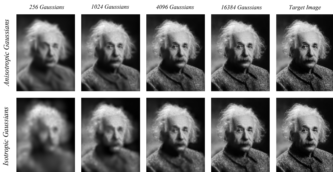
Figure 4: Image decomposition into anisotropic Gaussians using Expectation Maximization and isotropic Gaussians using Capacity Constrained Voronoi Tessellation ‡
