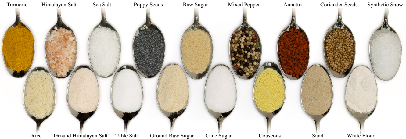
Figure 2: The appearance of real granular materials varies with the size, shape, packing rate, and scattering properties of individual grains.
