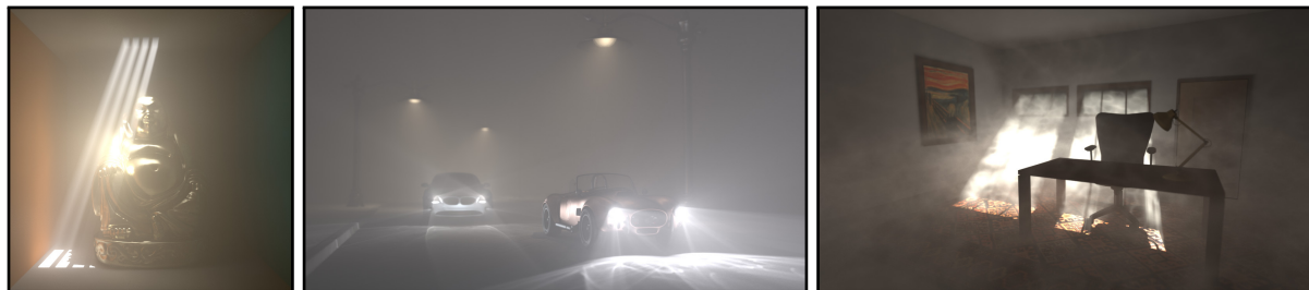
Figure 10: Full global illumination for the BUDDHA, CARS, and SMOKYROOM scenes, including the sum of the four components from Figures 7 and 9 as well as caustics computed using progressive photon beams and progressive photon mapping.
