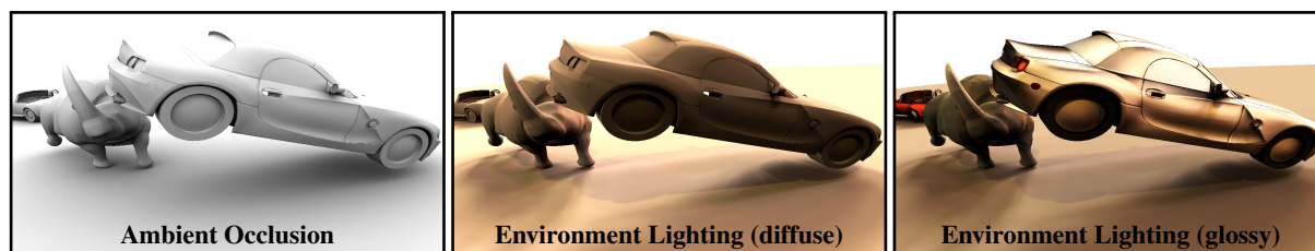
Figure 1: We compute spherical integrals of visibility-masked functions commonly found in rendering, e.g. in ambient occlusion and all-frequency direct illumination. This scene (123.2k triangles) took \sim 5 minutes to render on a 4-core CPU, independent of the lighting. These results render at 84% to 106% the speed of a noise-free ray-traced image, depending on the lighting.
