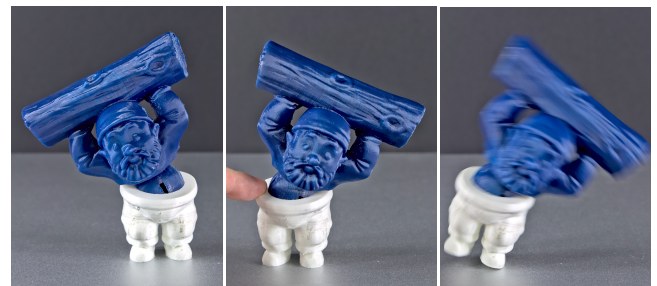
Figure 8: The Muscle Gnome is an example of an articulated model. Though the two poses look symmetric, the model stands stable when brought into the left-tilted pose but tips over in the right-tilted pose.
