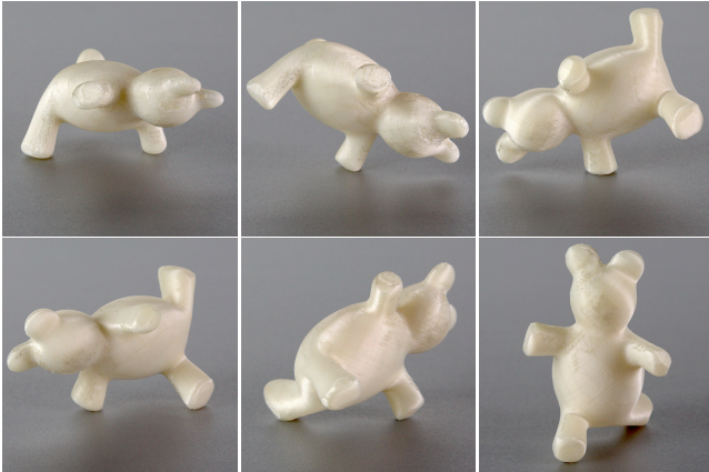
Figure 6: Using only two capsules we can optimize the Breakdancing Teddy to stand steadily in six surprising orientations.
