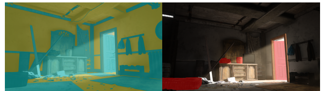
Fig. 2. We use different types of lighting representation in the same scene. On the left is a breakdown of models that use LLGs (teal) and geometry that uses lightmaps (yellow). On the right we highlight dynamic objects in red. Note that dynamic objects still use LLGs, hence the rendering pipeline is unaware of the difference. ©Activision Publishing, Inc.
