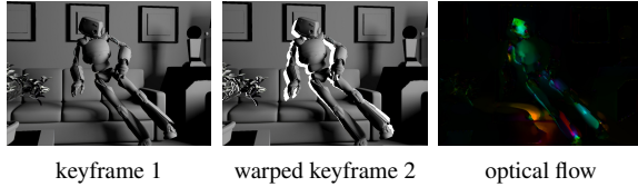
Figure 7: Optical flow-based motion estimation for the irradiance component (left). Using the primary motion vectors (Figure 4), we perform a motion compensation by warping the second keyframe (middle) where white pixels mark occlusions. The resulting flow (right) is added to the primary motion vectors to obtain the final motion estimate.
