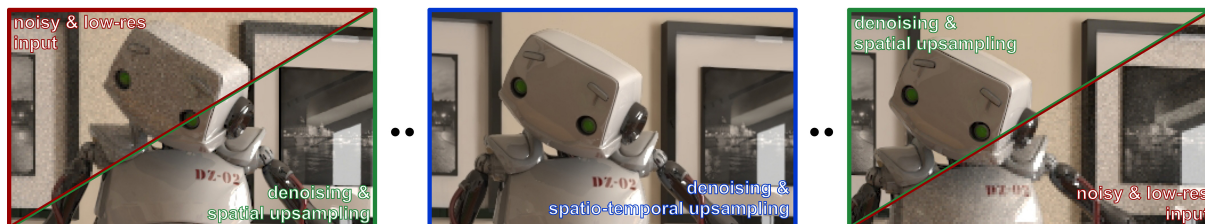
Figure 1: Starting from noisy, low-resolution frames generated with a path tracer (red borders), our method improves quality and reduces computational cost by computing spatially and temporally upsampled and denoised frames (green and blue borders) while properly preserving view-dependent shading effects like the reflections in the picture frame and on the robot.
