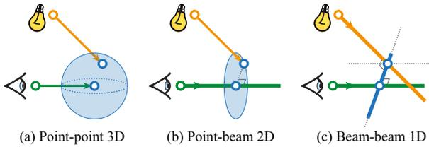
**Figure 10:** Different volumetric photon density estimators and their corresponding kernel (i.e. blur) dimensionalities.
