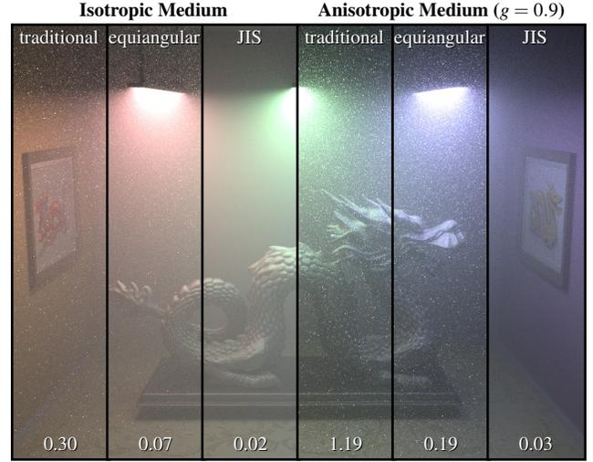
**Figure 8:** Single and double scattering in isotropic (left, 15 min.) and anisotropic (right, 30 min.) media rendered with unidirectional path tracing. Compared are light-source connections done via traditional transmittance-based distance sampling, equiangular distance sampling, and 3-random-decision joint importance sampling (JIS). RMS error is shown at the bottom. Figure reproduced from [GKH\*13].
