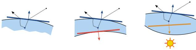
**Figure 14:** Illustration of random-walk-biasing schemes inspired by Dwivedi. Left: fitting a local slab to escape the volume close to the point of entry works well for thick volumes. Center: finding the closest surface point at every internal scattering point and biasing towards the surface point can help escaping thin geometric features. Right: explicitly biasing towards a light source improves backlit scenarios. Figure reproduced from [MHD16].
