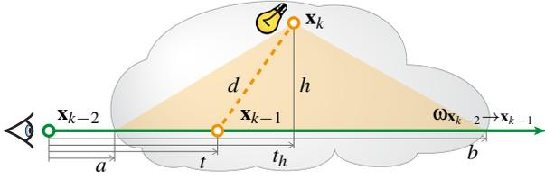
**Figure 6:** Equiangular sampling places points proportional to  $1/d^2$ , here limited to segment  $(a, b)$ .
