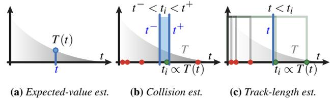
**Figure 4:** Expected-value estimators (a) calculate the transmittance value exactly. Collision (b) and track-length (c) estimators utilize free-path sampling techniques and check if the sample falls within an interval centered at  $t$ , or past  $t$ , respectively. Figure reproduced from [BJ17].
