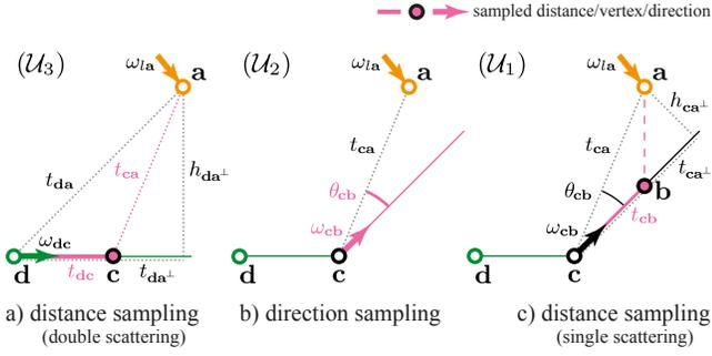
**Figure 7:** Given a point with an incident direction,  $(\mathbf{a}, \omega_{\mathbf{a}})$ , and a ray  $(\mathbf{d}, \omega_{\mathbf{dc}})$ , joint importance sampling constructs a 2-vertex connection with a prescribed joint distribution which can be factorized into a series of distance, direction and distance sampling decisions. Figure reproduced from [GKH\*13].
