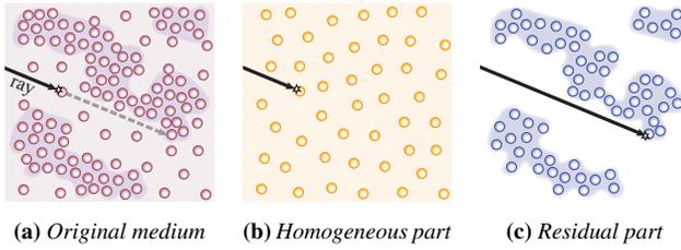
**Figure 3:** Decomposition tracking splits a heterogeneous medium into a homogeneous component and a residual heterogeneous component. The method then (lazily) samples free paths independently in each component and takes the shorter as the free path in the original medium. Figure reproduced from [KHLN17].
