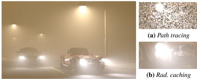
**Figure 13:** A scene with a fog rendered using 175K cache points and 27M cache queries with volumetric radiance caching [JDZJ08]. The insets provide an equal-time comparison to path tracing. Images reproduced from [JDZJ08].
