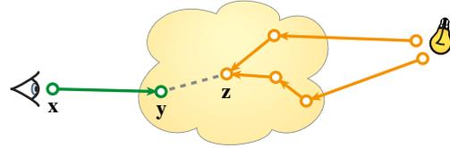
**Figure 16:** A difficulty with BDPT and emissive media. Accounting for the emission at the interior path vertex  $z$  requires evaluating a marginal PDF, which involves integration over all possible light subpaths arriving at  $z$  (colored in orange).
