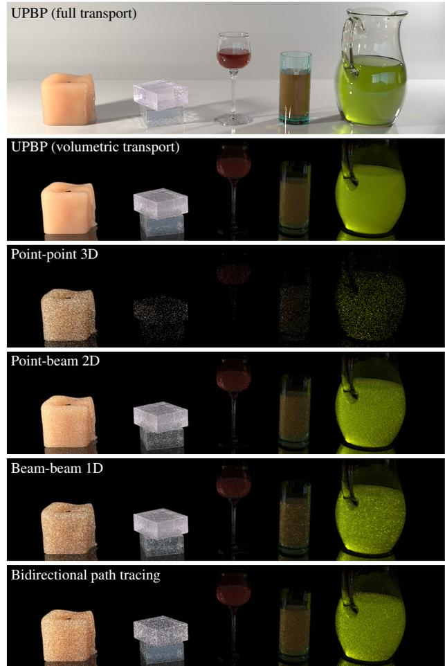
**Figure 11:** Equal-time comparison of UPBP against BDPT and the individual density estimators illustrated in Figure 10, showing that the combined algorithm can be significantly more efficient than each of its components alone. Images reproduced from [KGH\* 14].
