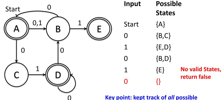
Key point: kept track of <u>all</u> possible States as input processed If <u>any</u> ending state is valid, then accept input
