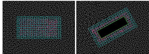
**Figure 9:** The consistency of SPH particles and FLIP particles in different reference frames. Left picture is a static reference frame without obstacle, right picture is the rotating reference frame with a rigid object.
