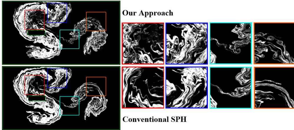
Figure 5: A paddle mixes smoke in a 2D box. The simulation results of our approach (top) and conventional SPH (bottom) are given respectively.
