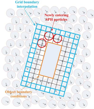
**Figure 3:** Three types of data transfer from SPH particles to the local FLIP solver.
