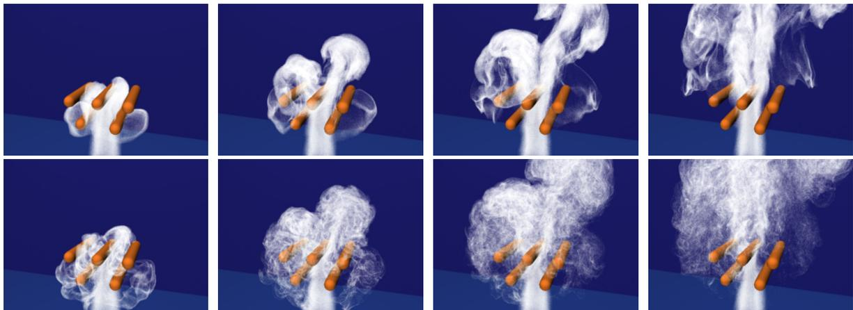
Figure 8: Rising smoke passes obstacles. Standard SPH (top) and our approach (bottom) are compared.
