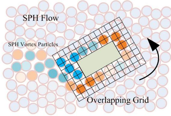
**Figure 2:** Method overview. Vortical details are created in the overlapping grid and preserved in SPH fluid. Different color represents the direction and magnitude of vorticity on each SPH vortex particle.
