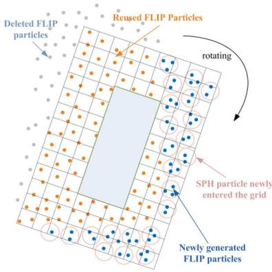
**Figure 4:** Seeding FLIP particles from SPH particles in the inner region.
