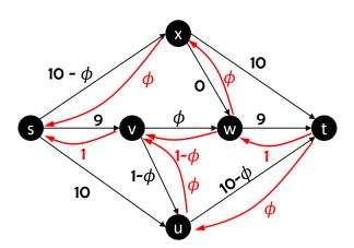
In Iteration 3, we provide the path (s, v, w, x, t). Note that  $\delta_3 = \phi$  again, and the current flow becomes  $F = 1 + 2\phi$ . After sending this, the residual network is (you are drawing first, right, and then checking?)
