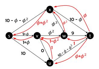
Note that the residual capacity of (x,w) is  $\phi - \phi^2 = \phi(1-\phi) = \phi^3$ .
