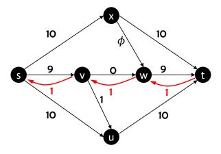
In Iteration 2, we provide the path (s,x,w,v,u,t). How much flow can we send on this path? Since  $\phi < 1$ , we see that  $\delta_2 := \phi$ . This makes the current value  $F = 1 + \phi$ . After sending this flow, the residual network is this (actually, draw it yourself and then check).
