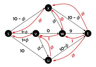
Now, in Iteration 4, we provide the path (s, x, w, v, u, t) again. The minimum  $u_f(e)$  edge is (v, u) with residual capacity  $\delta_4 := 1 - \phi = \phi^2$ . The value of  $F = 1 + 2\phi + \phi^2$ . After augmenting  $\phi^2$  flow on this path, we get the following residual network.
