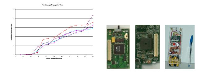
Figure 3: (Left) Path propagation time for 5 different paths over a grid of 54 Mote sensors. The y axis shows the time and the x axis the percentage of the sensors that are on the path and have seen the path message. (Center) A Mote board and Mote sensor board. (Right) The Flashlight device.
