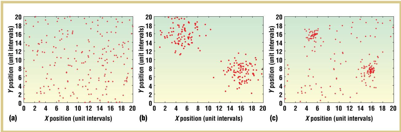
Figure 1. The results of a mobile-sensor simulation using a history-free update rule (with  $\alpha = 0.06$ ,  $\beta = 3$ ,  $\gamma = 1$ ): (a) the initial sensor positions, generated at random; (b) the positions of a series of 200 events; and (c) the final sensor positions.
