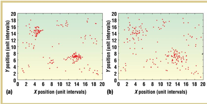
Figure 4. Results of a mobile-sensor simulation under the history-based algorithm: (a) the final positions of the sensors without noise and (b) the final positions of the sensors with noise of 25 percent deviation for each motion.
