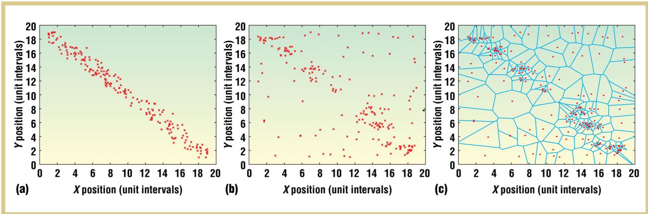
Figure 6. Representative results of predictive coverage maintenance: (a) event positions; (b) final sensor positions; and (c) a Voronoi diagram of sensor positions.
