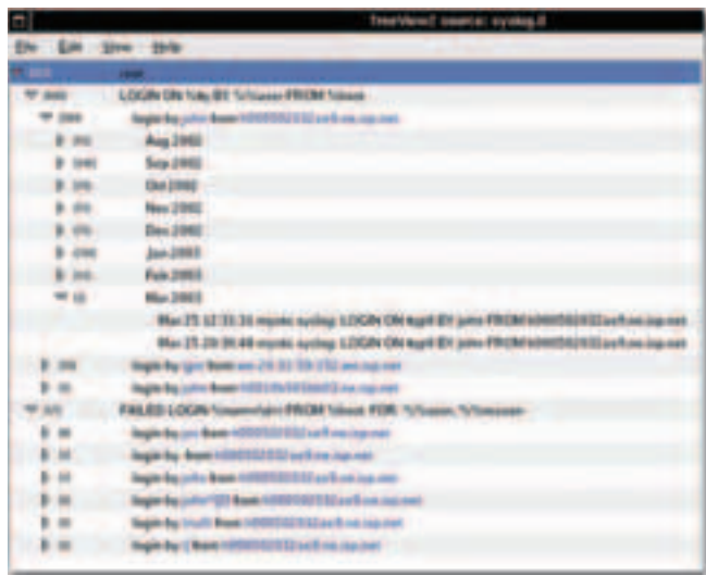
Figure 5. Treeview, some nodes expanded. The Kerf module for adaptive display of query results chose this summarization of the 600+ login events from *.isp.net.
