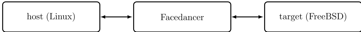
Figure 6.1: Diagram of testing setup. Software (in this case, umap) running on the “testing host” (left) causes the Facedancer to emulate a variety of USB devices when connected to the “target” (right).
