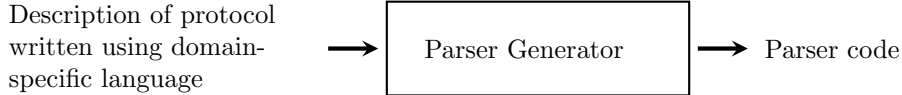
Figure 1.3: Workflow of a DSL-based parser generator. Given a description of the protocol language written in the domain-specific language, the parser generator produces the parser code.
