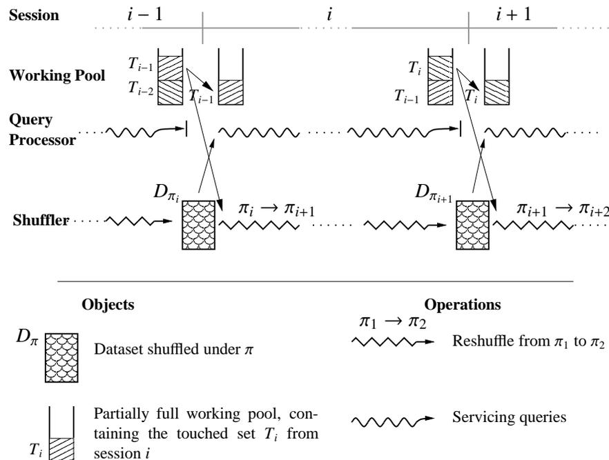
Figure 2. A snapshot of the overall algorithm across one session. At the end of session  $i - 1$  the shuffler has prepared  $D_{\pi_i}$ , and the query SCOP has a working pool containing the touched sets  $T_{i-1}$  and  $T_{i-2}$  (see Section 3.2). Then, the shuffler begins a reshuffle with permutation  $\pi_{i+1}$  and with touched set  $T_{i-1}$ . The query SCOP begins a new session  $i$  with  $T_{i-1}$  in its working pool, and filling in its own  $T_i$ .
