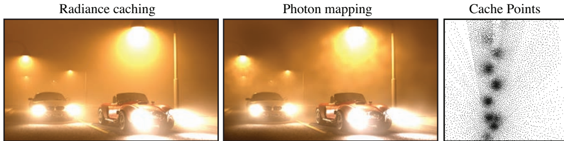
Figure 5.16: A equal-time, contrast-enhanced comparison between radiance caching and photon mapping in the cars scene from Figure 5.15. The scene has a large extent, making it difficult to render with methods such as photon mapping that compute scattering in the entire medium. Artifacts remain in the homogeneous medium even after storing 8M photons. On the right we show a horizontal cross section of the single scattering cache points as seen from above. In this visualization, the camera is located at the bottom looking up. Note the concentration of cache points around the street lights and headlights near the camera. The error tolerances were set at 0.25 and 0.75 for the single and multiple scattering caches, respectively.
