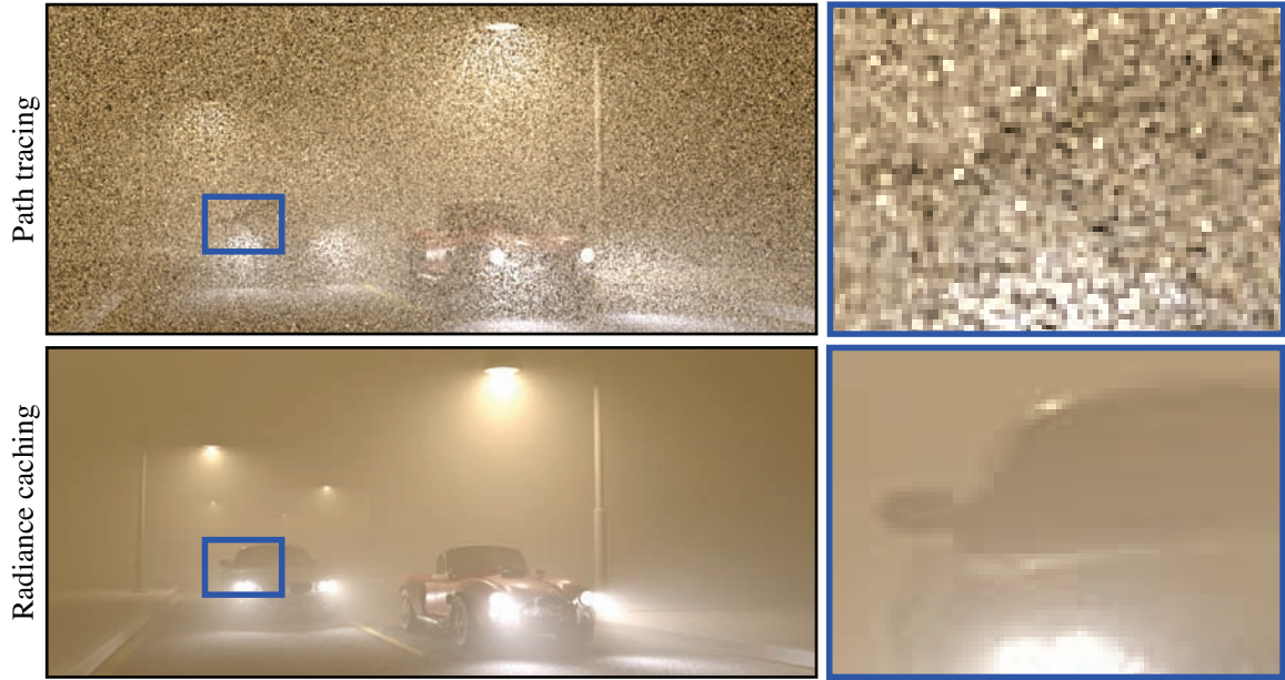
Figure 5.15: Two cars in a dense fog on a road illuminated by 60 lights. Our radiance caching method renders the cars scene in 20.35 minutes using only 175K cache points and 27M cache queries. The multiple scattering computation traces 4K random-walk paths per cache point. The highlighted region is shown zoomed-in on the right, providing an equal-time quality comparison between radiance caching and path tracing. The error tolerances were set at 0.25 and 0.75 for the single and multiple scattering caches, respectively.
