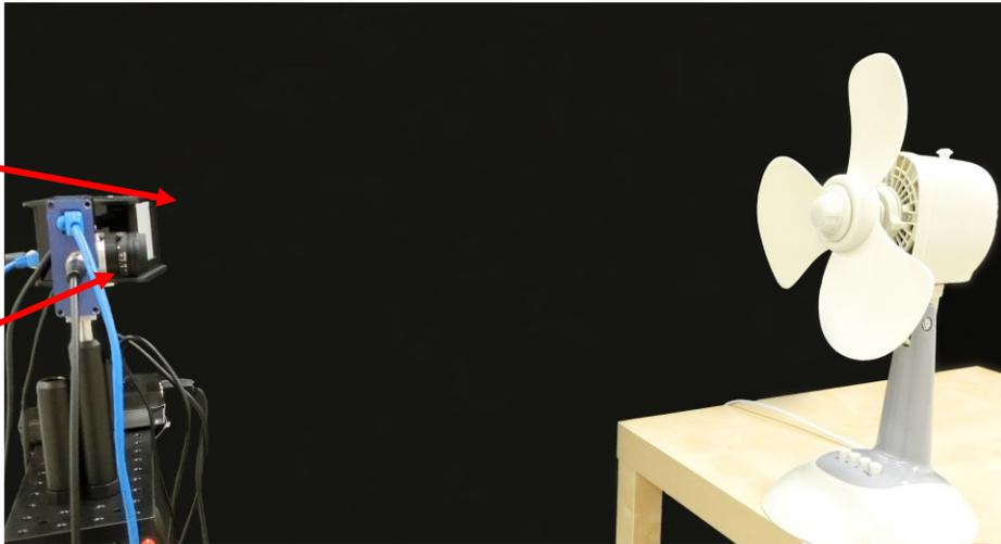
Imaging system setup for D-ToF camera
