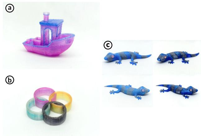
**Figure 8: Samples of multi-color objects printed using our inking device. (a) Two-color print of a Benchy boat. (b) Four-color print of overlapping rings. (c) Three-color lizard printed in opaque white PLA (left) and translucent PLA (right).**
