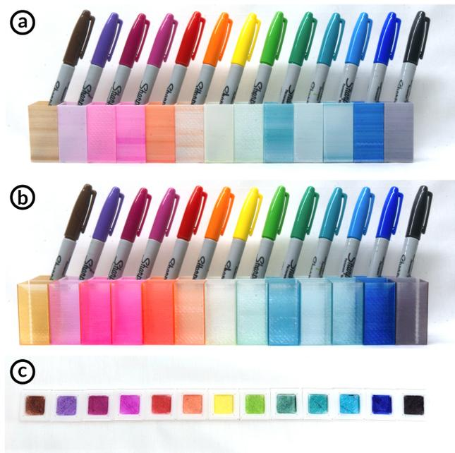
**Figure 7: A comparison of color reproduction using 13 different colored permanent markers on 3D printed objects. (a) and (b) show the color results of ink applied to filament prior to 3D printing. (c) shows the color results of ink applied after 3D printing. Filaments used: (a) opaque white PLA, (b) translucent PLA, and (c) opaque white PLA.**
