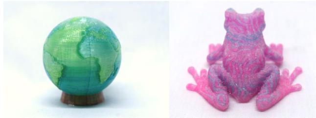
**Figure 9: Examples of color shifting when filament is not properly lined up with the GCODE executed by the 3D printer. Globe and tree frog prints retain distinct colors though shifted throughout the print.**
