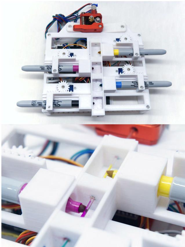
**Figure 3: Our inking device loaded with cyan, magenta, yellow, and black permanent markers, inking translucent PLA filament.**
