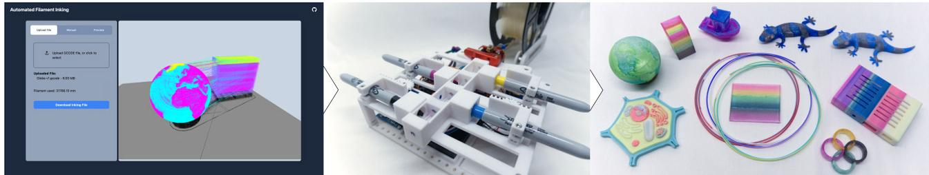
**Figure 1: Automated filament inking is a novel system for producing multi-color 3D prints with an FFF printer. Shown is a collection of multi-color 3D prints created using our open-source low-cost inking device and web interface for producing custom filament profiles.**
