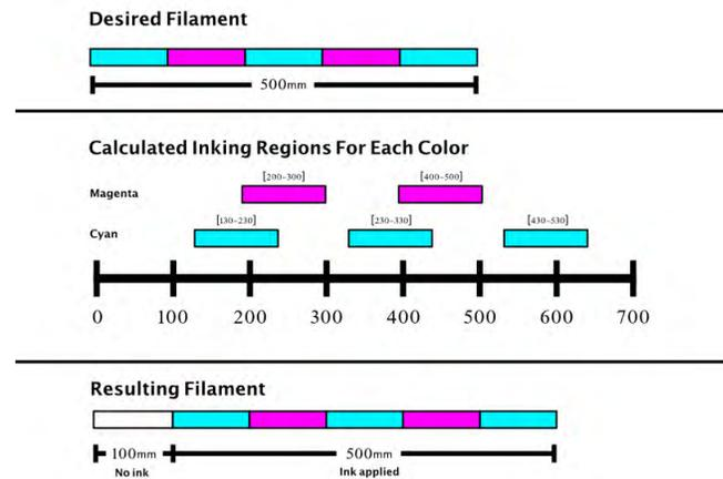
**Figure 4: Permanent markers on our inking device are spaced 30 mm apart, changing the regions in which each servo motor is engaged for coloring filament. An initial region of filament is left uncolored to compensate for the distance from the extruder to the last permanent marker.**
