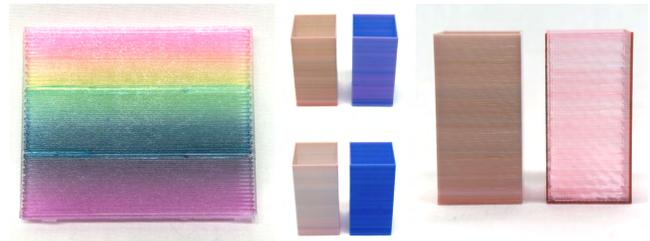
**Figure 11: Color mixing samples producing varying effects; rainbow gradients made using CMYK color mixing (left), directionally dependent prints where certain colors appear stronger from different angles (middle), and mixing differences between opaque and translucent materials (right).**
