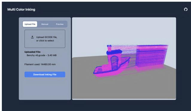
**Figure 6: A screenshot our web interface with built in custom GCODE viewer for visualizing the outcome of a multi-color print.**
