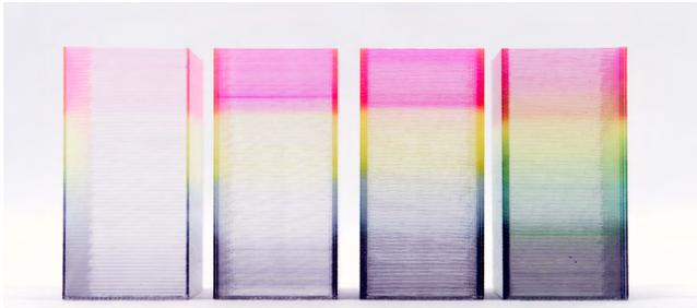
**Figure 10: Sample of spiral vase mode prints using translucent PLA colored with black, cyan, yellow, and magenta inks with increasing perimeter counts. The number of perimeters in a print affects the strength of the perceived color. From left to right: single perimeter, two perimeters and three perimeters with no ink overlap, and three perimeters with 200 mm of ink region overlap between colors.**
