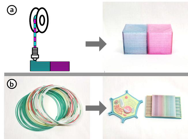
**Figure 5: Illustrations of inked filament becoming a 3D object. (a) Alternating regions of inked filament results in the conjoined cyan and magenta cubes. (b) Complex multi-color objects require varying regions of inked filament.**
