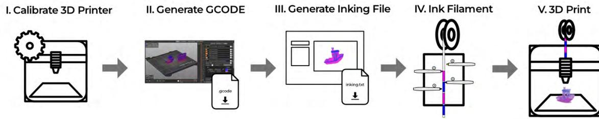
**Figure 2: The workflow of our five step process for multi-color 3D printing. The steps include calibration of the printer, generating GCODE for the 3D printer, generating the inking.txt file for the inking device, inking filament with the device, and 3D printing with the filament and the GCODE file.**
