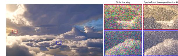
**Figure 1:** A cloudscape rendered with a combination of our spectral and decomposition tracking techniques, which gracefully handle chromatic media and reduce collision coefficient evaluations. The insets on the right were computed in equal time, with our method yielding 3.5x lower MSE than delta tracking.
