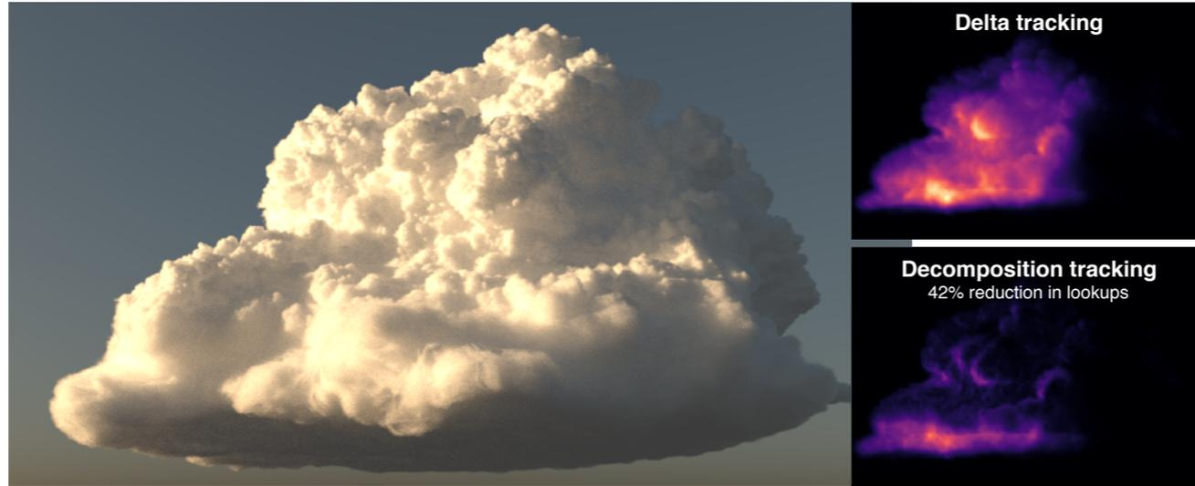
Here is an example. The cloud was subdivided using an octree where each cell contains a homogeneous and a residual heterogeneous component. Decomposition tracking reduces the number of extinction lookups by 42% yielding the same free-path samples as delta tracking.
