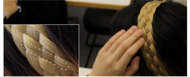
**Figure 9** A user performs a subtle swipe gesture on a braided head band to interact with a computing device.
