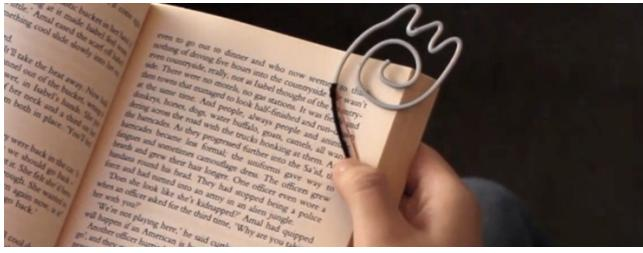
Figure 11 When reading, a user uses the interactive tulip bookmark to control ambient light.
