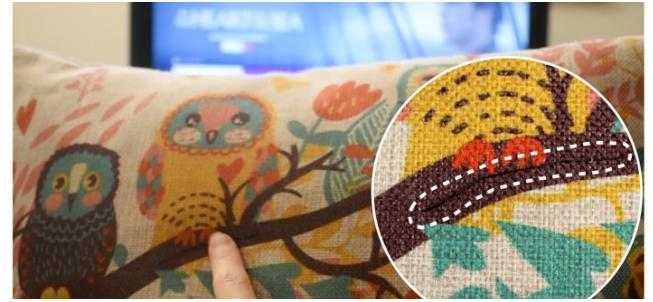
**Figure 10** A user control the TV program using touch input on ThreadSense, hand-sewed on a cushion.
