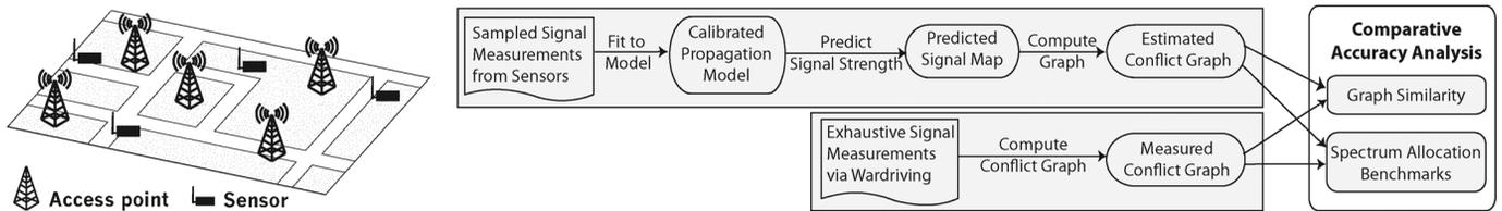
Fig. 1. Our high-level methodology. We build *estimated conflict graphs* using a small number of signal measurements at randomly selected locations. We use these samples to calibrate a propagation model, predict signal strength values, and construct conflict graphs. We examine the accuracy of estimated conflict graphs by comparing them to *measured conflict graphs* built from exhaustive signal measurements, using graph similarity and spectrum allocation benchmarks.
