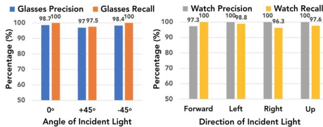
Figure 14: Accuracy of gesture recognition under ambient light in varying directions.
