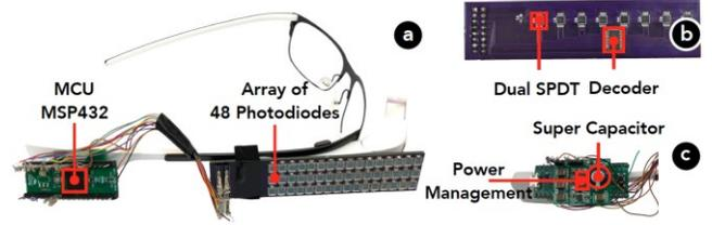
Figure 7: Integrating the prototype with Google Glass.
