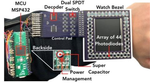
Figure 8: Integrating the prototype with a smart watch.
