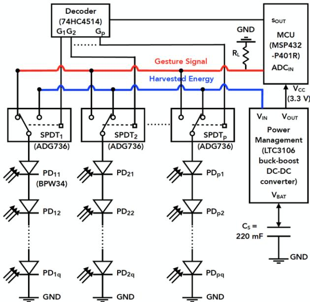
**Figure 9: Schematic of our prototype, where  $q$  photodiodes are wired in series as a group connecting to a switch, and  $p$  photodiode groups are wired in parallel, connecting to the power management, decoder, and micro-controller.**
