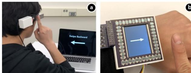
**Figure 1: Integrating our prototype with a glasses frame (a) and a watch (b), where arrays of photodiodes harvest energy while being reused for sensing finger gestures.**
