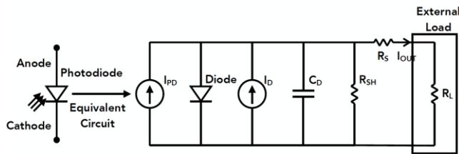
Figure 2: Equivalent circuit of a junction photodiode.
